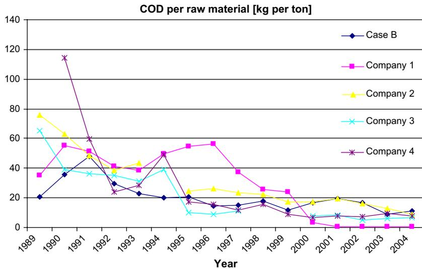
Fig. 5. COD emissions per ton raw material at five herring processing industries [11,14,21,22].
