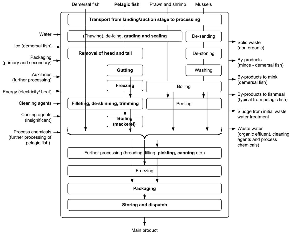
Fig. 1. Different processes and overview of the main categories of inputs and outputs of the four main product categories (or product chains) in the Danish fish processing industry [16]. The product chains investigated in this article are written in bold-faced type.
