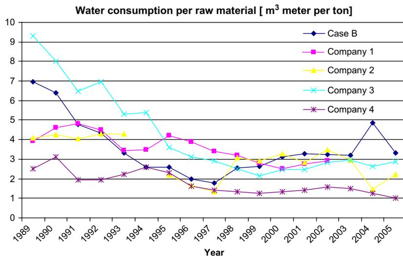
Fig. 6. Water consumption per ton raw material at five herring processing industries [11,14,21,22].
